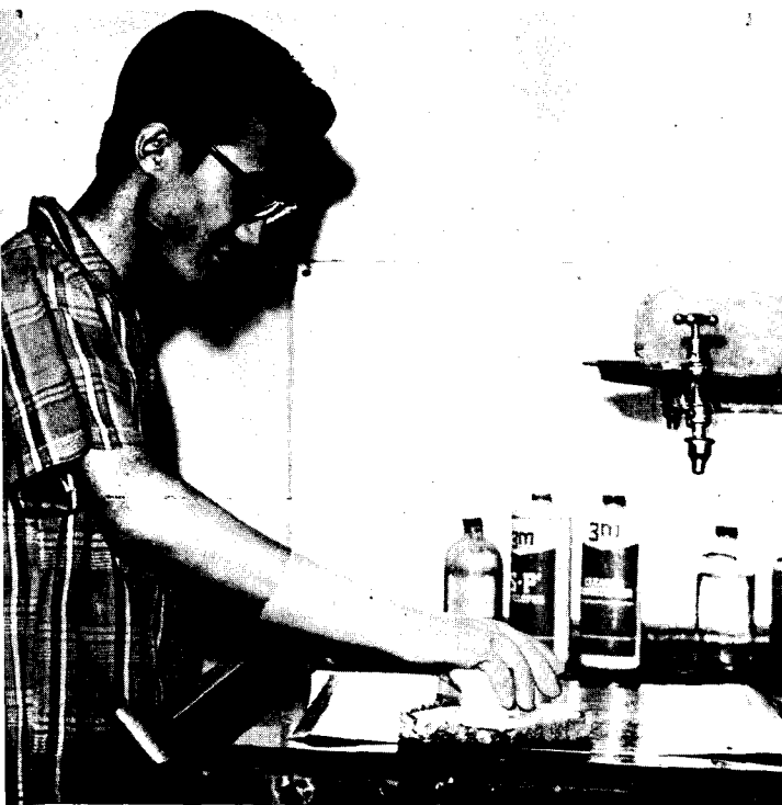
PLATEMAKING. The approved "masters" are placed on sensitized aluminium plates in a vacuum printing frame. Ultraviolet light exposes the parts without words or pictures. The exposed plates are developed, fixed, inked and gummed by P. A. Tan.
