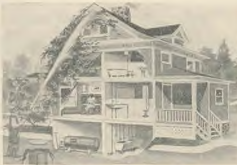
Kewanee Water Supply Outfit in Operation
