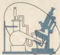
▶ This microphotometer is used for measuring the intensity of the spectrum lines obtained on photo plates when using the spectrograph.
