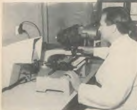
▶ A technician uses a spectrograph. The ash of opium is placed in the cavity of a carbon electrode and exposed to direct electric current.
