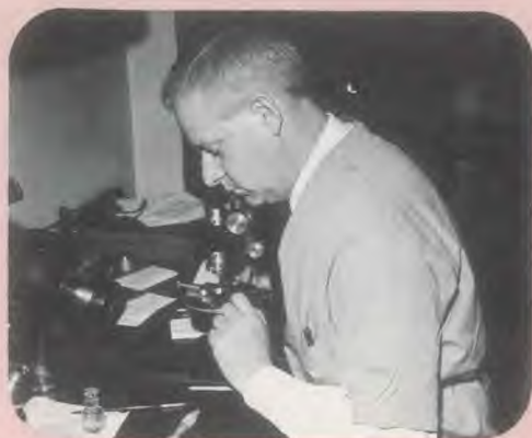
A 210-power polarizing microscope, which can be used to compare crystalline structures of unknown tablets with known, to identify them.
