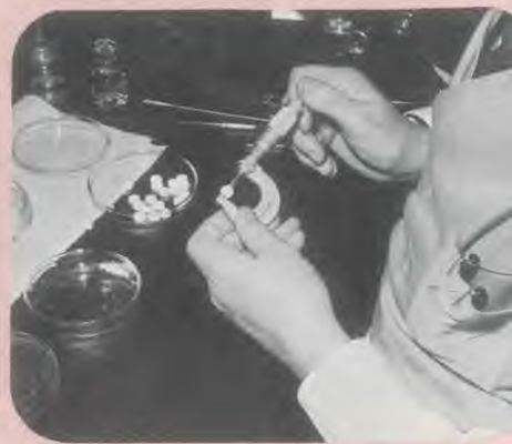
With a micrometer, an investigator measures the exact dimensions of a tablet being tested in order to make sure it meets established specifications.
