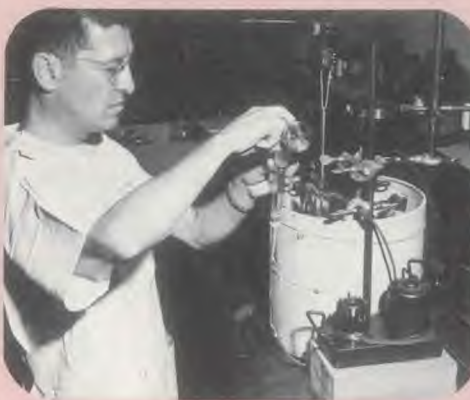
This "artificial stomach" tests a dextroamphetamine tablet, by determining the rate of its dissolution under the simulated conditions of digestion.
