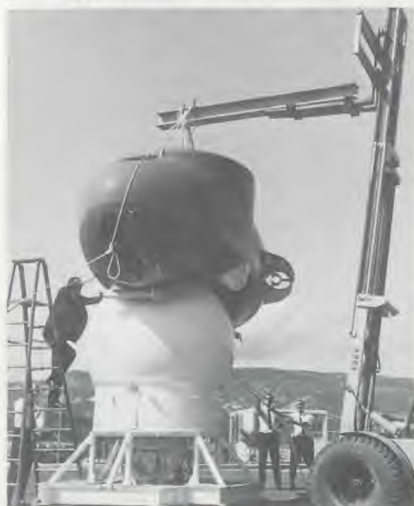
LAB FOR OCEAN DEPTHS. The eight-inch pressure sphere of a two-man deep-ocean work boat receives its tight-fitting fairing. The sphere is designed for use at depths of 6,500 feet.
