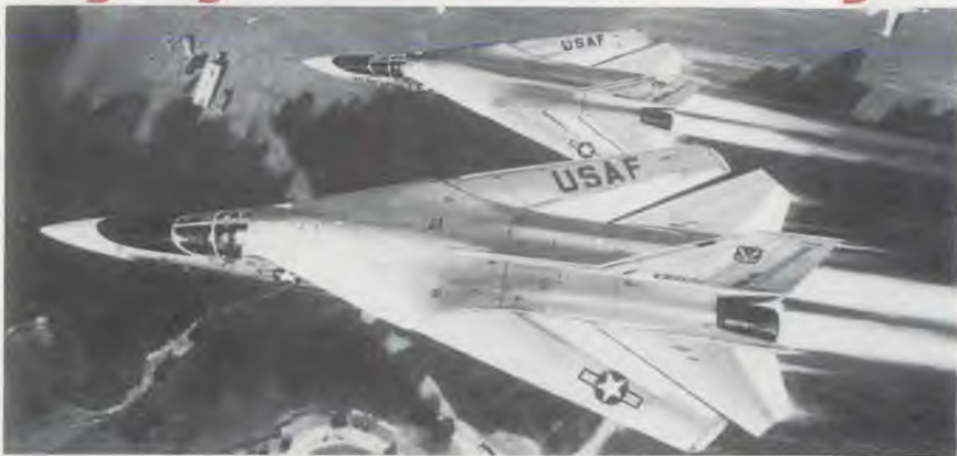
Air Force's F-111 displays its chief design asset, the wings that sweep back into a thin triangle for supersonic flight, then stretch out to provide more lift on takeoff and landing.
