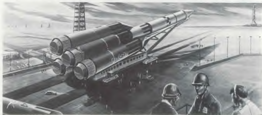
CALLING FLIGHT NO. 1 FOR SATURN. Future launch vehicles for interplanetary missions may be built on a "cluster" principle, according to a report by Douglas Aircraft Company engineers. Liquid-propellant vehicles would be preferable for launching large pay loads. A booster with four clusters would have 45.5 million pounds of thrust; five external boosters would provide a maximum thrust of nearly 55 million pounds.
