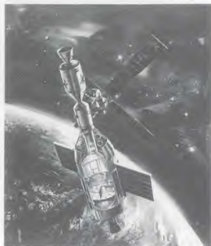
This space workshop will enable astronauts of the future to work in a shirt-sleeve environment. The "wings," panels of solar cells to provide electric power, are folded down during launch and extended after orbit is achieved.
