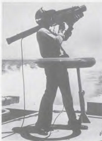
REDEYE MISSILE designed to strike low-flying aircraft is tested for shipboard use at Pacific Missile Range, Point Mugu, California.
