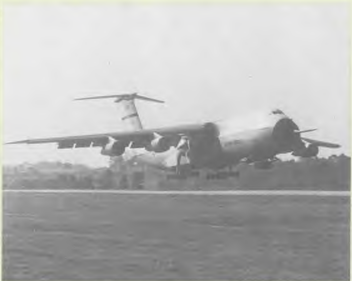
HISTORIC FLIGHT —U.S. Air Force/Lockheed C-5 Galaxy, largest airplane ever built, spreads her 223-foot-span wings and flies for the first time. The 728,000-pound transport is 268 feet long and has a normal maximum payload of 110 tons. Under emergency operating conditions payload can increase to 132 tons.
