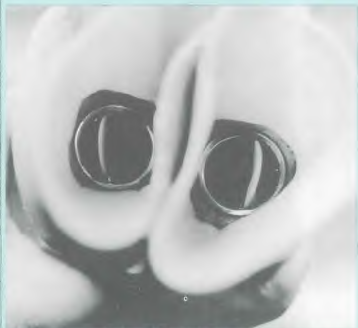
Closeup view of the valves of the Orthotopic Cardiac Prosthesis, a mechanical device used as the first total replacement of a human heart.
