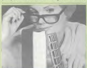
This experimental communications device, smaller than a standard textbook, has a built-in special-purpose computer that makes possible the transmission of high-speed data on conventional telephone lines.
