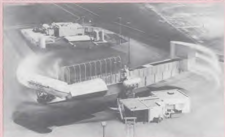
Groups of four space engineers spend from eight hours to seven days as test crewmen inside the gondola on this giant spinner at this space center in California. The tests will provide information for the construction of an earth-orbiting space station planned for the 1970's. The spinning creates an artificial gravity similar to that of a rotating space station.
