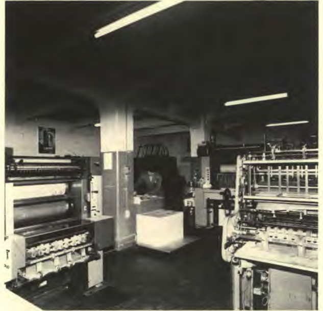
In a space that should accommodate no more than two presses there are five. This makes it difficult to carry the paper to each of the machines as it is needed.
