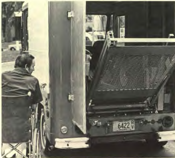
With a push of the button Ed Beaudoin can lower an access gate to his new van.
