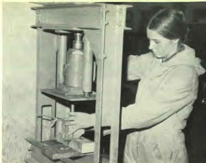
Top, Julie Rorabeck seats a wrist pin in a piston. Left, Neville Watson removes the oil pan on his project. Opposite page, top, Auto mechanics students in the classroom disassemble and trace down the idle system, intermediate system and the high-speed system in the carburetor. Bottom, James Nash, center, assists two students in checking specifications for timing degree and dwell angle.
