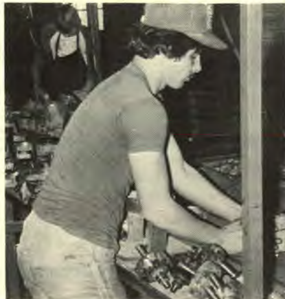
Crates of old alternators arrive by the truckload. Students dismantle them and sort and label the parts.
