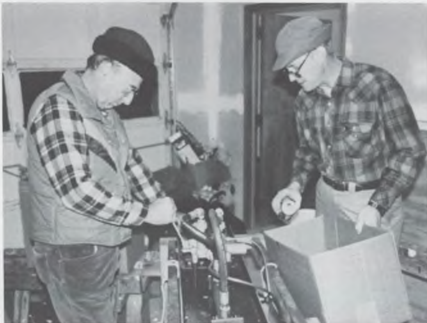
Bill Jeffries (left) and Hilman Culp working at the hydraulic aluminum-can smasher they designed and built. Previously cans were crushed manually.
