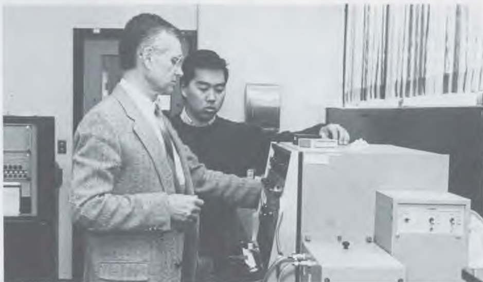
In one of Roger Pak's chemistry classes, he learns how to measure light absorption intensity in a compound using a spectrophotometer. Dr. Wilkins, left, assists. Photos by Brad Leavelle.
