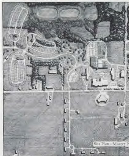
The master site plan shows a proposed location for the auditorium-fitness center and three proposed sites for cabins, recreational vehicles and tents with a bathhouse at each of the three sites.
