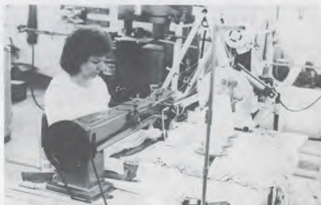
Carol Hainey pulls yarn from several spools, cuts and then stitches on the "Consew" sewing machine to create the mop.
