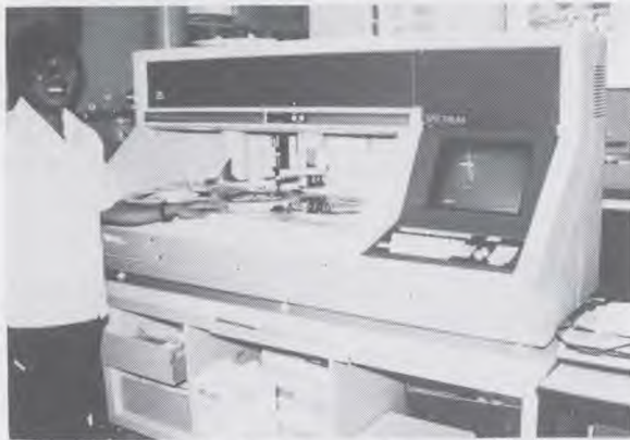
Spectrum Biochemical Analyser - This computerized machine is the state of the art in analysis of numerous biochemical parameters. It can perform over 20 different biochemical estimations simultaneously on each blood sample.
