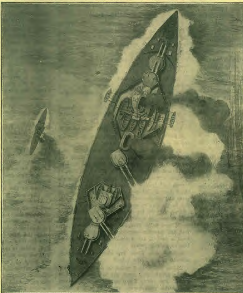
The Monarch, England's latest improved war-ship of the Dreadnought type. She carries but one military mast, and is so built that she has the least possible superstructure, so that "every scrap of unnecessary gear may be done away with." She can fire a broadside of ten 13.5 guns, each projectile weighing 1,250 pounds. She has a displacement of 22,500 tons, and 27,000 horse-power. Her small boats, two of which are shown in the cut in the act of being launched, are provided with "shelter screens," so that they may be protected from the fire of the enemy.
