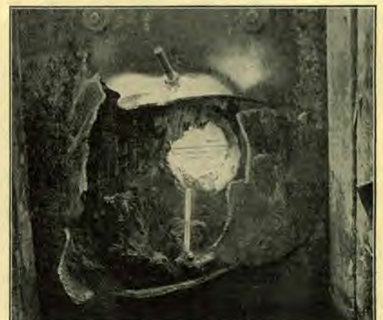
A hole made through an 18-inch Krupp armor-plate and its timber backing, by a shell from a 12-inch gun
