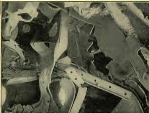
Wreckage and distortion at the back of an 11½-inch armor-plate, made by a bursting shell that has passed through it
