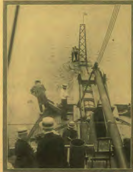
International Jules Verne's dream of exploration beneath the sea is to be realized in still another submarine apparatus. Simon Lake has invented a boat—the Argosy-Argonaut—with this strange looking caudate appendage—a thirty-foot steel tube, terminating in a steel chamber eight feet long, seven feet high, and seven feet wide at the bottom. In operation, the chamber is lowered until the bottom rests upon the floor of the ocean; and by means of compressed air, men may enter the tube, descend to the chamber, and walk along on the sea bed. A larger craft with a tube 300 feet long is being built, with which it is intended to salvage some of the many sunken treasures lying off the eastern coasts of America.
