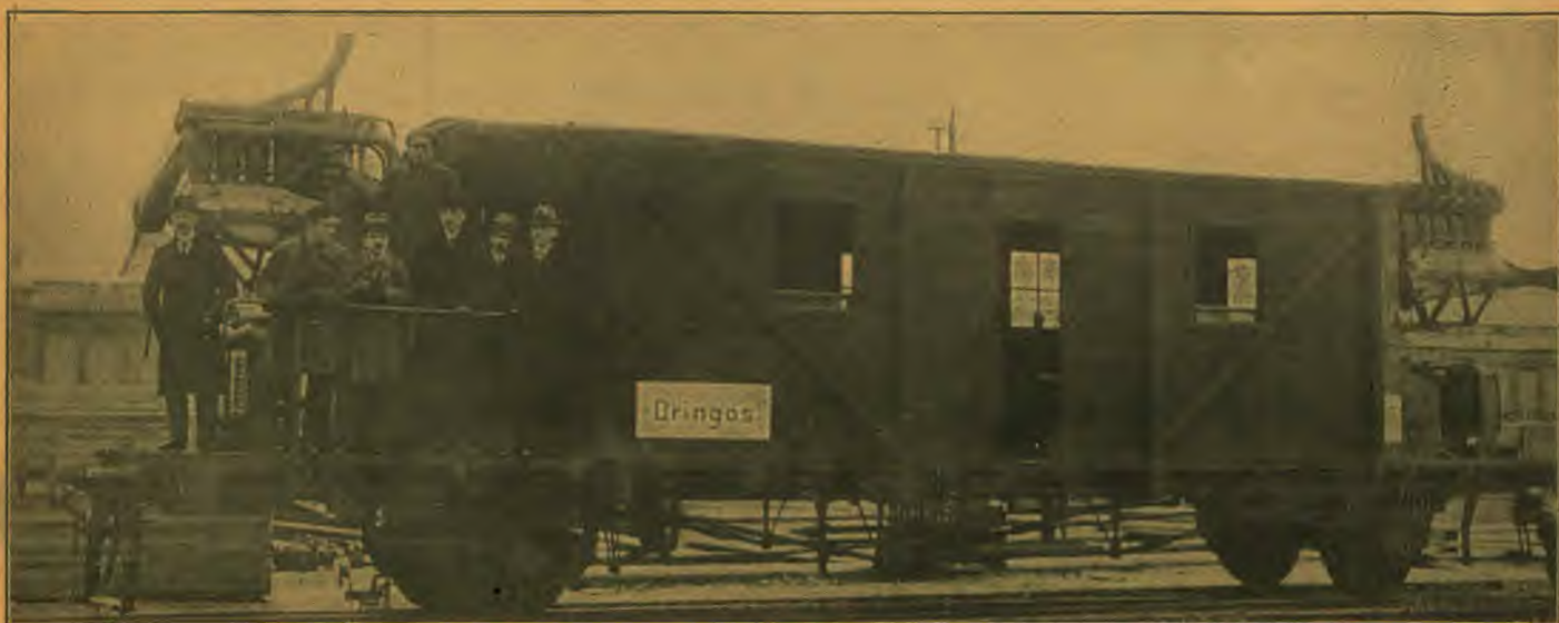
Dr. Otto Steinitz, of Germany, has discovered a new use for aero propellers. This car is reported to have covered the distance between Berlin and Hamburg, 300 kilometers, or 186.3 miles, in one hour, or an average of over three miles a minute. The motors are of 160 horsepower each. The saving in fuel by this method of propulsion is said to be considerable. It is quite possible that such an adaptation may displace the steam locomotive in many places, as electricity has done already.
