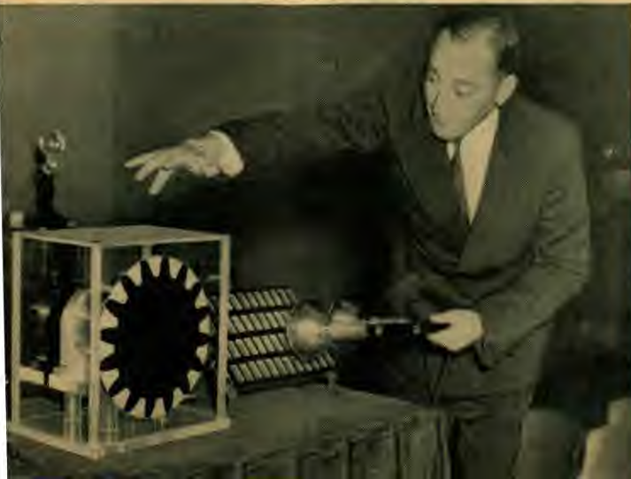
Demonstration of a sun motor in General Electric's exhibit at the New York World's Fair. The disk is driven by a motor that derives its power solely from electric energy converted from light.
