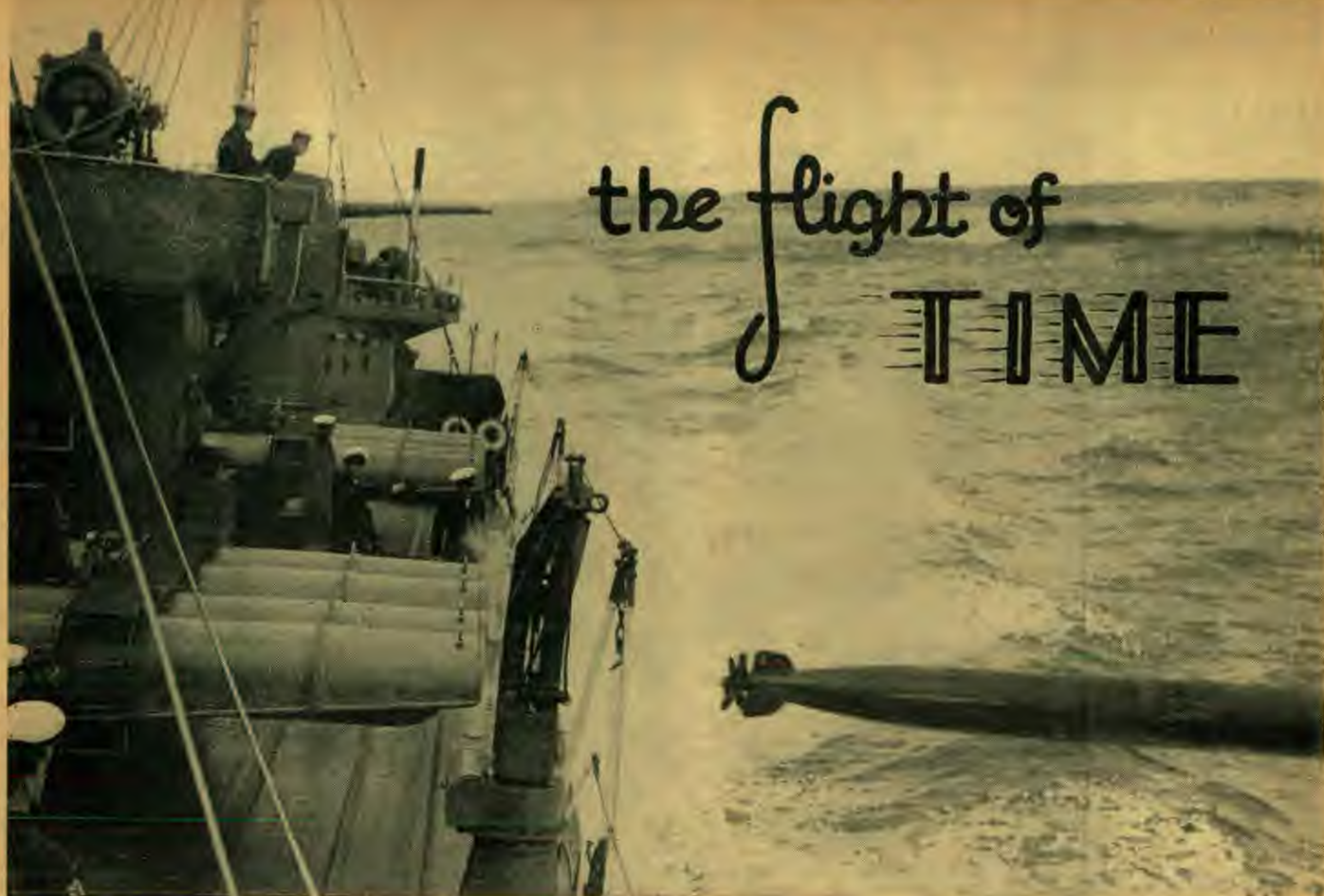
INTERNATIONAL A torpedo at the moment of launching from a French cruiser. Compressed air "fires" the torpedo, which proceeds under the power of its own motor after entering the water.
