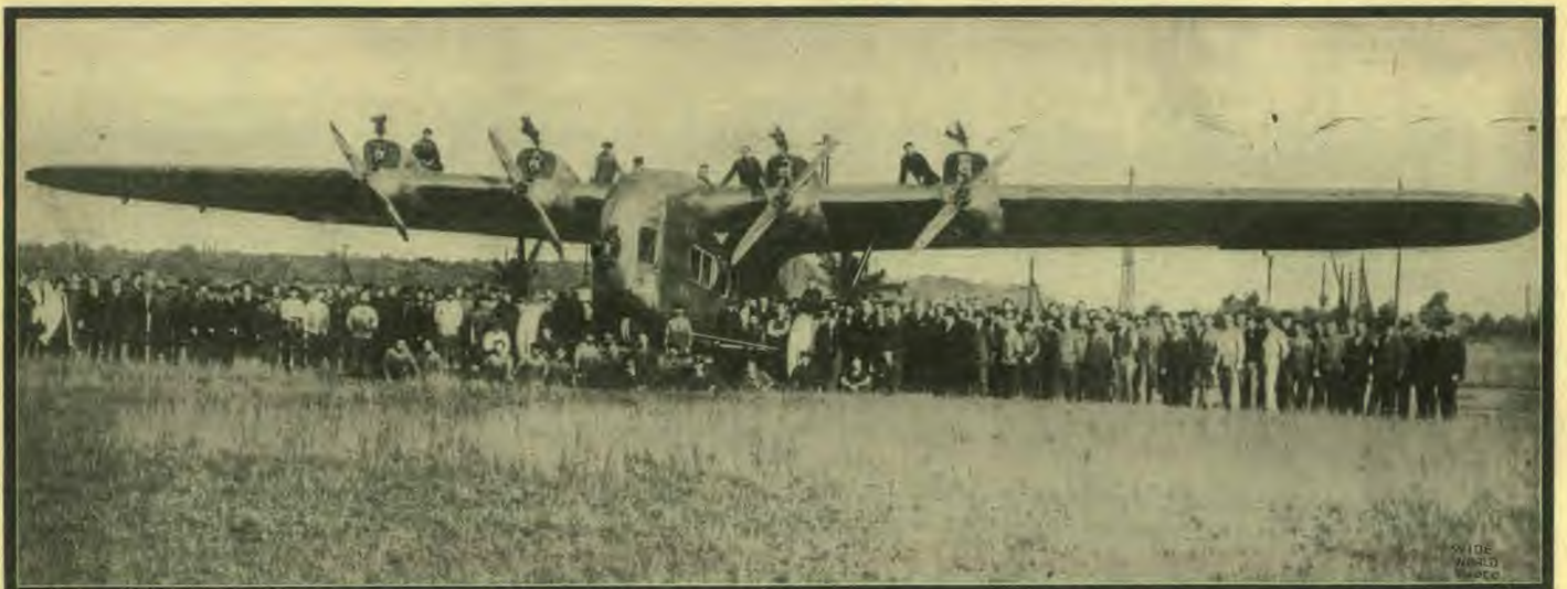
The newest type of passenger plane has recently been put out by the Staaken aëroplane factory in Germany. The plane is made of aluminum entirely, and is of the monoplane type. Its four engines, each of 250 horse power, are built in the wing of the plane instead of in the fuselage. It carries eighteen passengers with all the comforts of a Pullman. Its wing spread is approximately one hundred feet, and it has a speed of 130 miles an hour.
