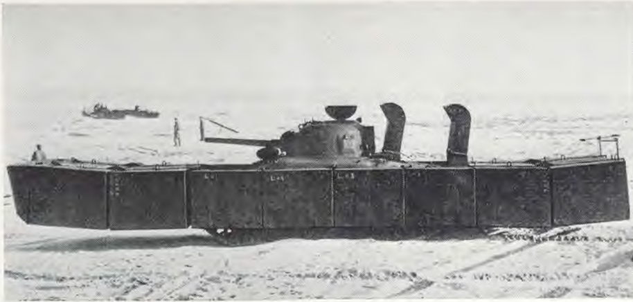
This strange monster of war is a device that permitted 30-ton tanks to be launched at sea to swim ashore at 5½ miles per hour, with guns blazing all the way. Once ashore, a member of the tank crew touched a button inside the vehicle and the rivets holding the pontoons fast exploded, freeing the tank of its "seagoing girdle," and permitting it to plunge forward unhindered. These tanks were first used at Okinawa. (Photo by Acme.)
