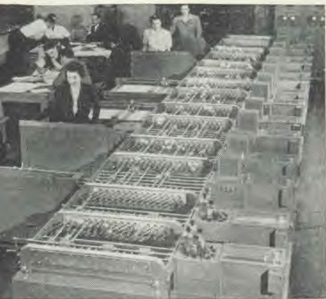
This mechanical wizard, which is at work at the General Electric plant at Schenectady, can work out mathematical problems in two weeks that would require seventeen man-years to accomplish.
