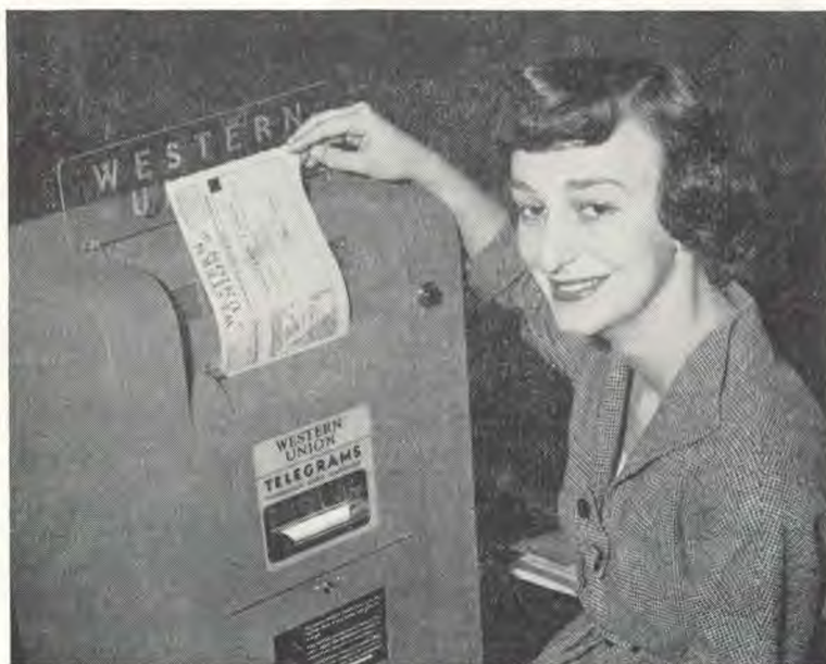
This new Western Union Telefax machine was installed recently in the Capitol. Drop telegrams into a slot, press a button, and automatically the telegrams are wrapped around a revolving cylinder. An electric eye scans them and flashes them over the wires, recording facsimiles at the terminal.
