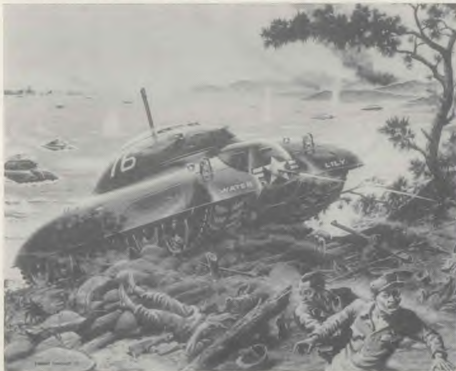
Technical engineers have designed this undersea tank for amphibious landings. Still in the blueprint stage, the tank offers a solution to the many problems in spearhead landing operations. It gives added protection against menacing underwater obstacles.
