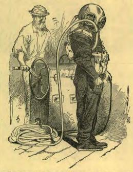
in the accompanying picture. The suit is made of India rubber, covered inside and out with tanned twill, to protect the rubber from injury. It is air-tight and water-tight. The helmet is made of tinned copper; the sleeves fit tight around the wrist, leaving the hands free; and to the soles of the shoes are attached heavy lead weights. Air is supplied by a force-pump, through a tube connected with the
