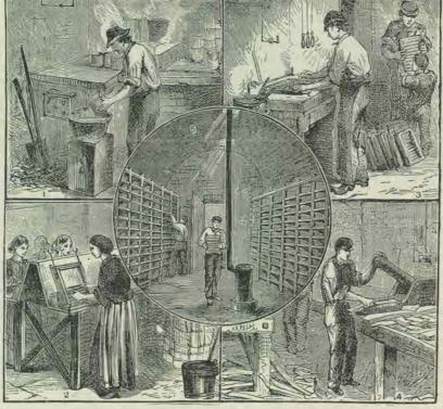
that make the matches. These fall in a shower from the machine, and are gathered, by an ingenious machine, into rings of iron, where they are held separate from each other, yet fastened tightly in the frame, and the ends of them are dipped into a solution.
