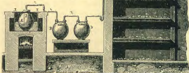
Apparatus for producing bleaching-powder by passing chlorine gas generated in A; upon quicklime spread upon the shelves
