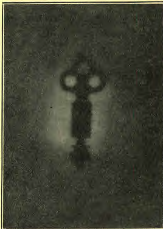
This picture was made by placing a key on the outside of a light-proof plate-holder containing a photographic plate. A block of radium-bearing ore three quarters of an inch thick was then placed on the key, and the photograph resulted.
