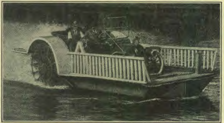
AUTOMOBILE IN PLACE FOR DRIVING BARGE ACROSS A BAY ON THE PACIFIC COAST
