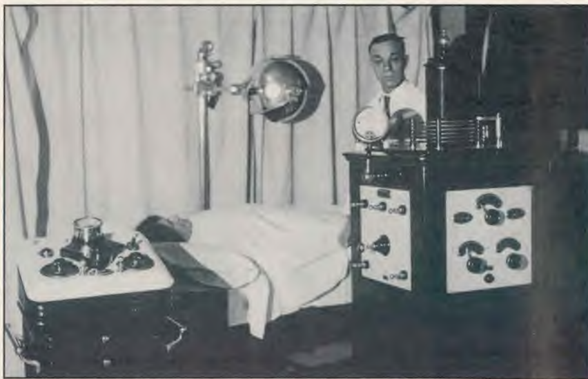
An example of an early diathermy treatment room at New England Memorial Hospital. This machine could warm the body tissues without damaging them through high-frequency electromagnetic radiation.
