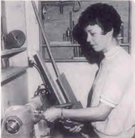
In basic woodworking class a student turns a coffee table leg on the lathe.
