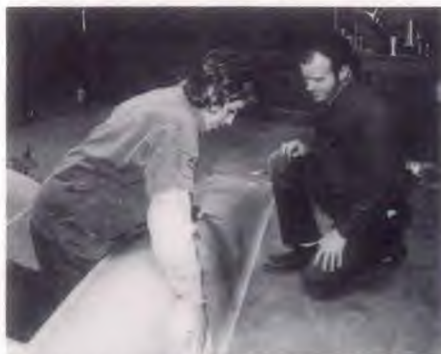
Two fiberglass students polish half a canoe just removed from the mold.
