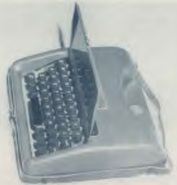
This machine makes it comparatively easy to visit with a blind-deaf person if he knows braille. You press the lettered keys on the front of the machine, and he feels the small metal pegs which respond in braille on the back where the shiny disc about the size of a quarter is located.
