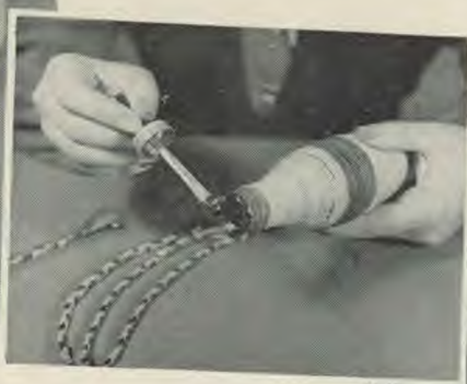
Figure 2. A Good Coat of Glue Goes on the Bottle Before Putting on the Braid
