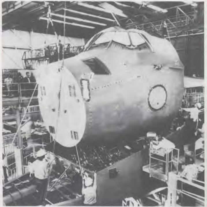
The crew compartment of the Space Shuttle Orbiter, which is to house the crew of what is hoped will be the nation's first reusable spacecraft, is installed into the shuttle's lower forward fuselage. Roll-out of the first orbiter is scheduled for this fall.
