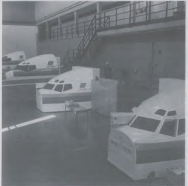
Here's a room full of electronic flight simulators, which exactly duplicate the controls of several different aircraft. A simulator can reproduce every known situation that may arise during actual flight, thus giving crews practice in working together—and meeting emergency situations—before getting in the air.
