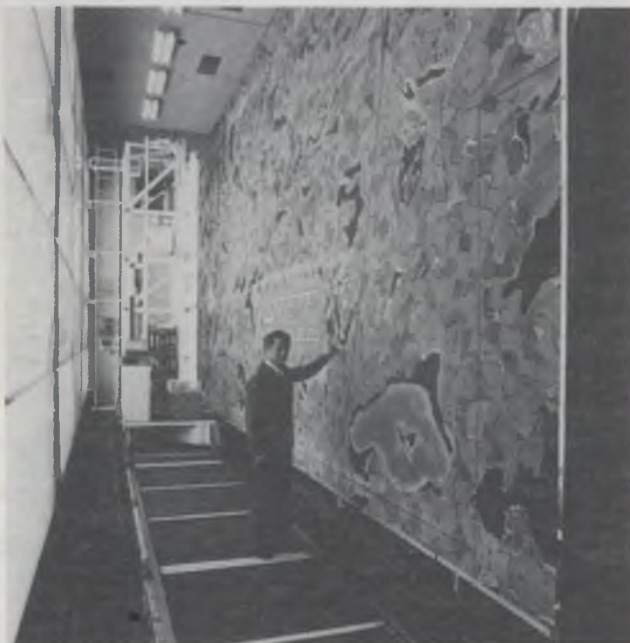
Ed is dwarfed as he stands beside the panorama that provides the visual system for the simulators. A special TV camera is mounted so that it can move across the panorama as the pilot "flies" the simulator around the landscape.
