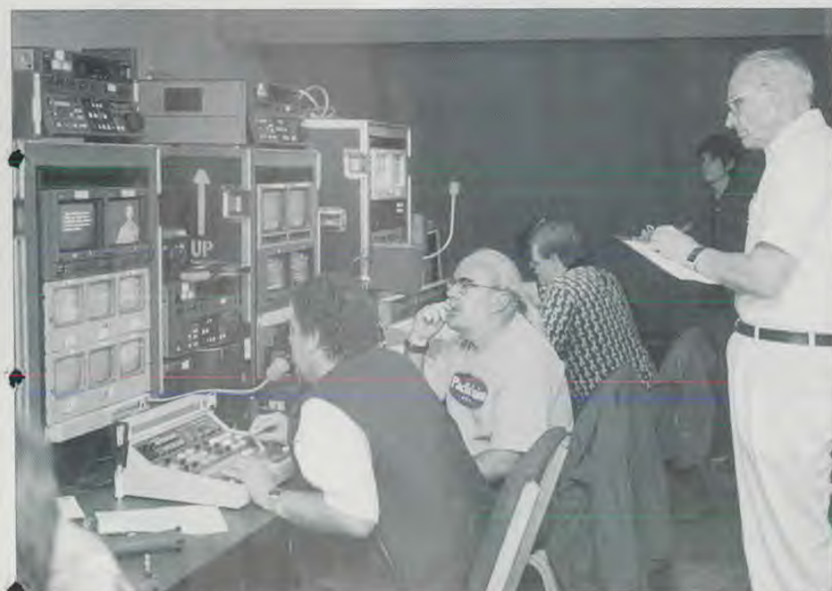
Professional technicians in the control room mix the many images from the video cameras with the computer-generated graphics to produce the final signal that goes out over the satellites to the down-link sites around the world.
