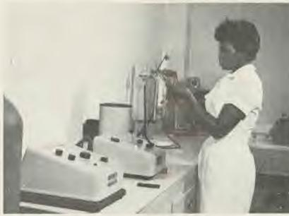
The modern laboratory includes this Coleman flame photometer and spectrometer, operated by Sarah High.
