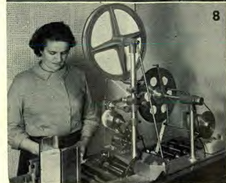
8. Model No. 301 Scriptomatic addressing machine imprints names and addresses from the cards onto address strips (7/8" wide tape) at the rate of 40,000 per hour.
