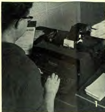
1. An electric typewriter types the name and address on the face of the card while special carbon reverses it on the back for imprinting.
