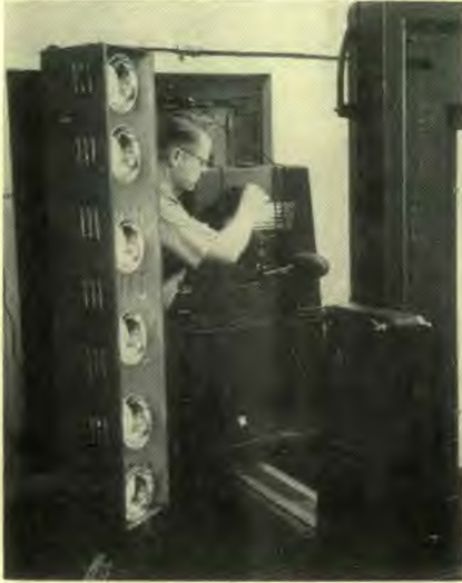
Mr. Farnsworth setting the diaphragm on the Brown process camera.
