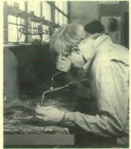
Oxyacetylene welding provides the student with a knowledge of the working characteristics of steel.
