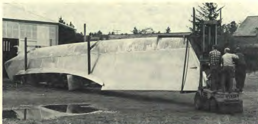
To counterweight the forklift while the hull is moved from the shop, workers stand on the back side. They include Jamie Spence, Bill Peterson, Al Bakke and Jimmy Rhone.
